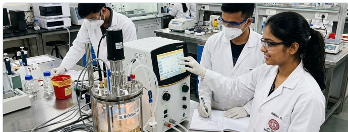
Bioprocess Engineering Suite: Students operating automated 5L stirred-tank bioreactors.
